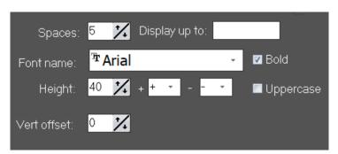
Each item part can be individually formatted; spaces before the item part, display up to, font and size vertical offset and for numerical values, positive, negative, up and down arrows.
