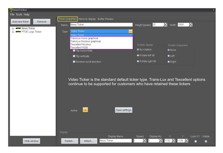
Within **Ticker Properties**, the standard ticker type is a **Video Ticker**. For a new user this type should be selected and it defaults to full colour with the **LED Colours** (checked).
