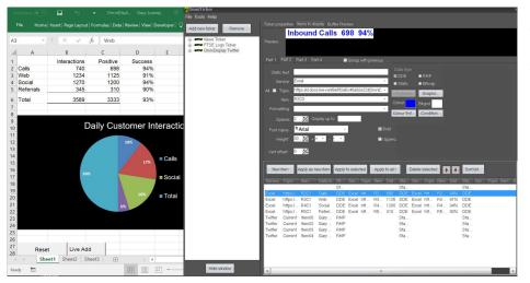
The Feed handler auto-connects to OmniRSS with a default port 5004. The message log records the applications actions and provides a user with any errors in attaching to the associated programs and services.
